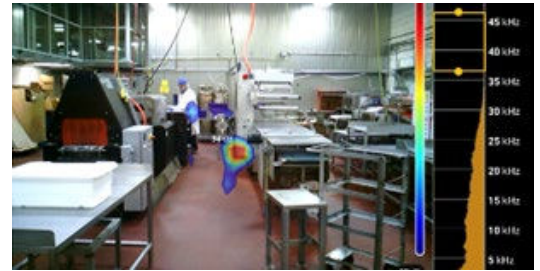
Above: Sonic imaging readout detects previously hard-to-access air leaks through SugarCreek's award-winning project.
